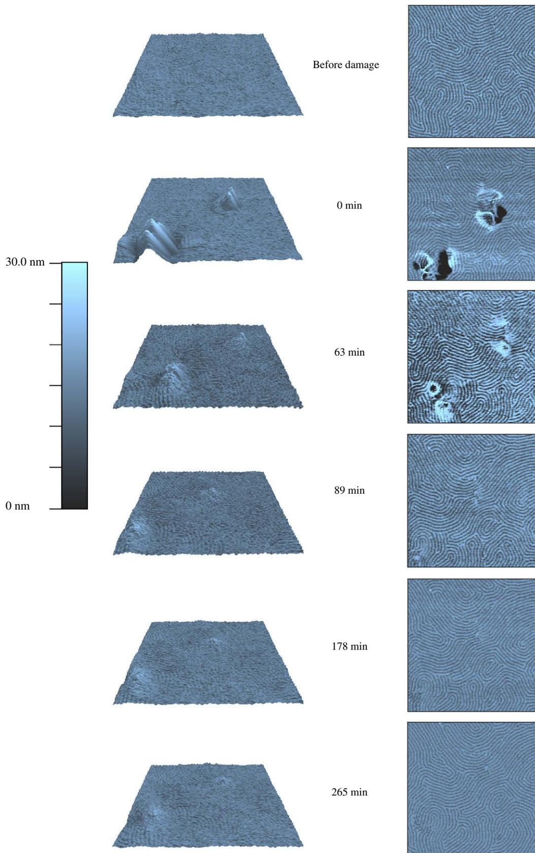
**Fig. 3.** AFM height (a) and corresponding phase (b) images of catastrophic polymer damage and healing, taken at 398 K. Note that the later-time phase images shows nearly-perfect recovery, while the height image shows a peak remaining. The flattening of the topographic peaks virtually stops after 90 min, just as the final fingerprint pattern is frozen in.
