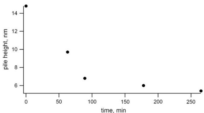
Fig. 4. The decay of the height of the tallest part of one of the peaks (the one on the right in Fig. 3) is shown as a function of time. This decay is non-linear: it proceeds more quickly at early times than at late times.
