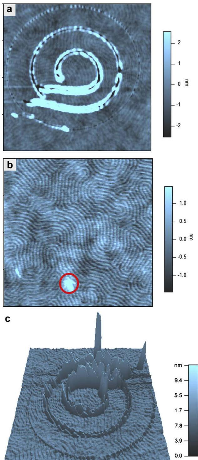
**Fig. 1.** Tapping height image of a  $2 \times 2 \mu\text{m}^2$  PS-*b*-PMMA before (a) and after (b) healing a scratch. The pattern was created using *MicroAngelo* software on an Asylum MFP-3D atomic force microscope. (c) 3-dimensional version of (a).
