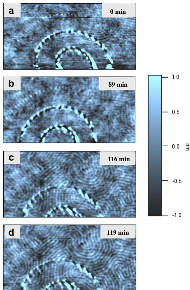
**Fig. 2.** A sequence of images showing the healing sequence of the bull's eye pattern. The scans are  $1 \times 2 \mu\text{m}^2$ , with the height scale of 2 nm. The temperature was ramped from room temperature to 373 K between 70 and 80 min into the experiment. Notice the outer ring vanishing at this temperature.
